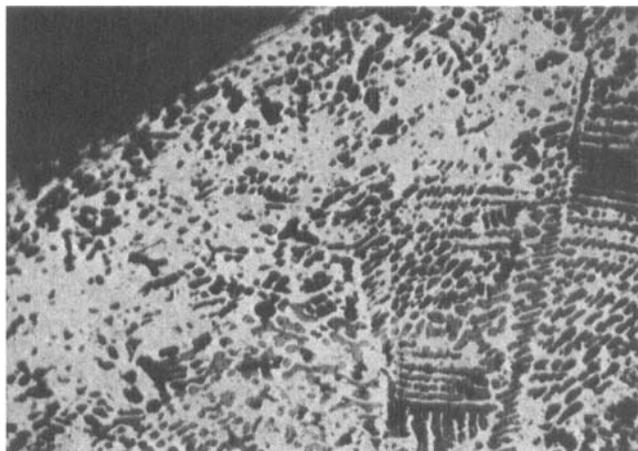
FIG. 2. Magnification  $\times 100$ . No metallographical attack. External part of an equatorial section of a partly oxidized denarius. Average percentage of silver at present: 59%. Percentage of silver in the central part (not visible on the negative): 49%. The pits appear in black, the copper grains appear in grey.
