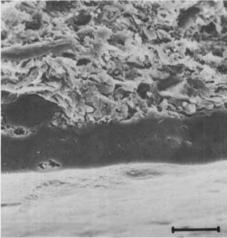
Plate 1 *Contact zone between the black coating and the porous sherd matrix. Sherd no. KP 1.6-3259/11.
